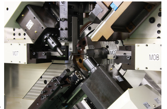
Upper/Lower tables travel 40mm from side to side Quill travels 60mm back-and-forth
