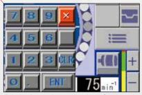
By utilizing the numerical keypad, one can set the corresponding counters, cam, or stroke counts.
