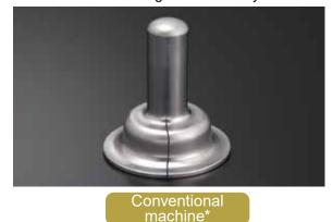
The conventional machine cracked the part in the final step.
