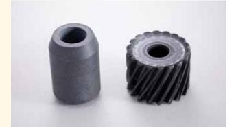
Before processingAfter processingSize:Size:Ø17.6 x Ø9.2 x 25.8 mmØ23.2 x Ø7.0 x 17.0 mm
