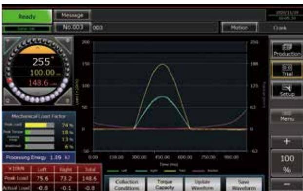
This screen displays the information necessary for trial production that repeats trial hitting, evaluation, and setting.
