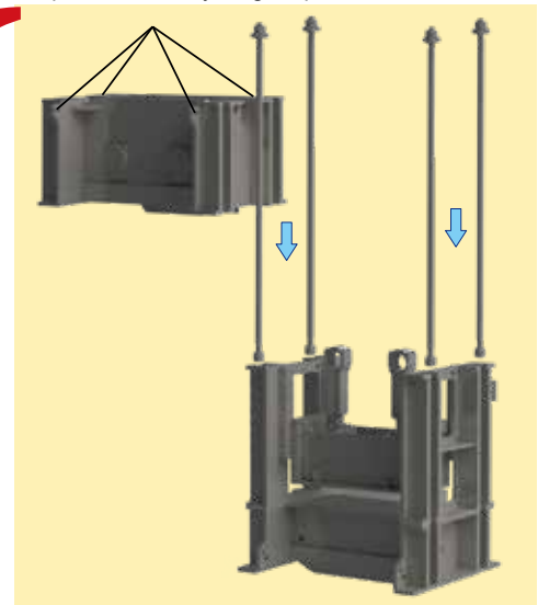
Conventional method: insert tie-rods from above
