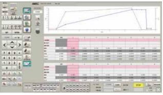
**Program for number of coils** (cylindrical coils) By freely inputting numerical values for the pitch and outer coil diameter, you can easily adjust the compression spring program.
