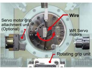
The rotating grip unit can be also used for long length forming.
